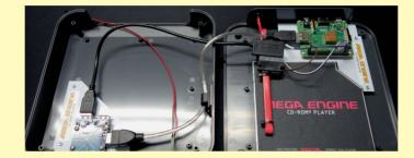
Now connect the wires from the power LED to pins 8 (VCC) and 14 (GND) of the Pi's pin header. The VCC pin of the power LED is again marked with a white stripe. Add a cable tie to the all the wires coming from the Pi's pin header (except the disc drive's ground wire) to clean up the install.
