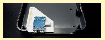
Then install the L-shaped carrier PCB into the bottom part of the case using the remaining three torx screws. Make sure the nuts on the bottom of the PCB are aligned straight with the PCBs edge. Start with the torx screw on the bottom left, then the one on the right and last the top one. Make sure the nuts actually sit inside the case and not on top of the case's edge. Then use the four 4mm long Phillips screws to attach the Pi3 SOC to the top of the spacers on the bottom PCB.
