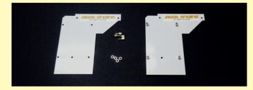
The triangular PCB is the top one. Use four Phillips screws (the 5mm long ones) and four washers to install the four F/F spacers as shown below in the middle. The washers go on the same side as the spacers. Then use the remaining four 5mm long Phillips screws to attach the USB expansion board on top of the spacers as shown.
