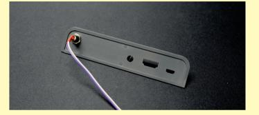
The pre-soldered white LED gets installed into the front panel. This is ideally done using a drop of hot glue or any other glue that you're comfortable using and doesn't take ages to harden. You will find the the top of the LED fits the hole perfectly, so it's easy to hold the LED in place while you wait for the glue to strengthen. This is the trickiest part of the whole build.
