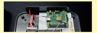
Put the front panel into place into the top part of the case, but do not yet connect the wires coming from the LED.
